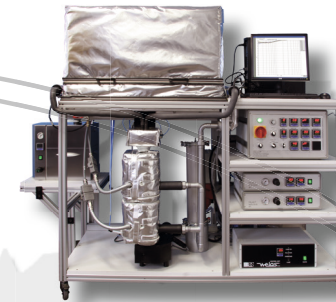
HMT 1000 for oil mist separators, blow-by, closed crankcase ventilation, isothermal, heatable, t \leq 130^\circ\text{C} \pm 200 mbar variable inlet pressure with welas® digital 1000
