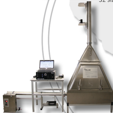
TVE 3000 / TVE 3000 S for vacuum cleaners according to EN 60312 with welas® digital 3000
