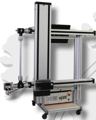
Traversing unit for filter leak tests with y = 700 mm and x = 1000 mm incl. software for scanning and leak analysis incl. welas digital 2000 measuring device 0.2 - 40 \mu\text{m} 32 size channels per decade
