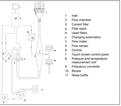
Figure 1: Design and operation flowchart
