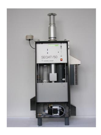
PM10- and PM2,5 STANDARD REFERENCE SAMPLER according to CEN EN 12341
