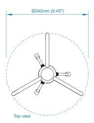
Positions for three off bolt fixings with Ø7.0mm (0.27") max. thread. on a p.c.d. of 85mm (3.35")
